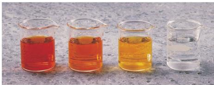
Figure 5. The decrease in Bromine Concentration Over Time is Visible As The Solution's Color Fades (From Left to Right).
